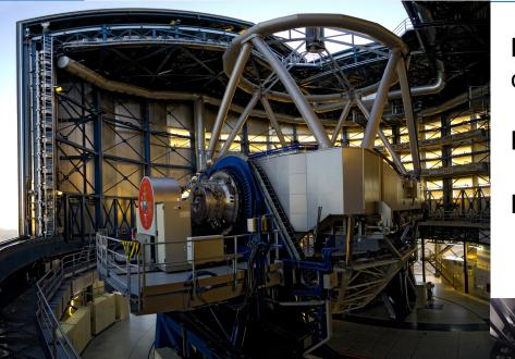
**M1**: 8.2m diameter (175mm thick), actively controlled by 150 actuators
