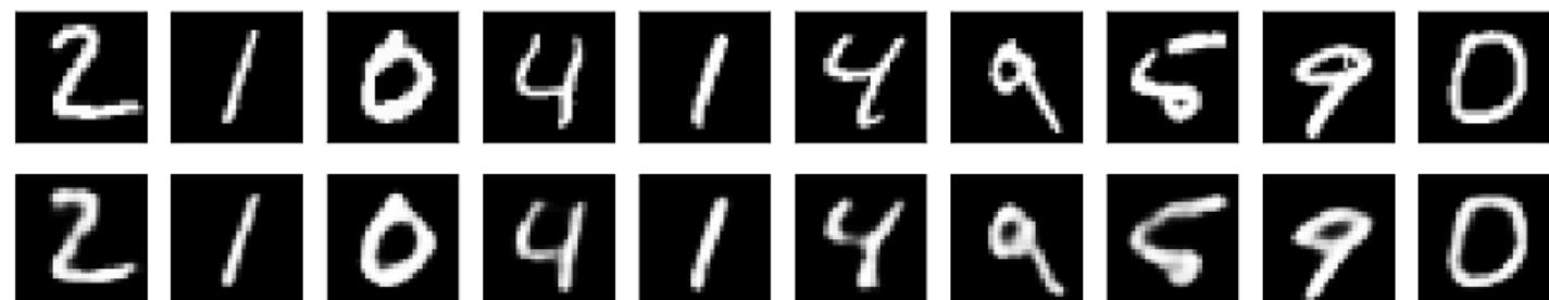
outputs of convolutional autoencoder with 8 layers of size  $4 \times 4$  in the latent space (128-dimensions)
