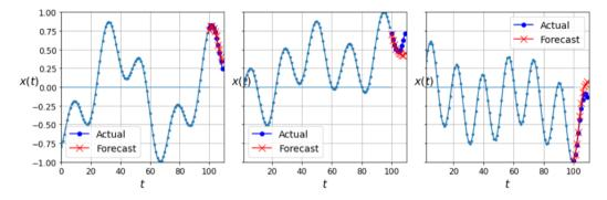
This is so far the best network. Its MSE is for last predicted point is 0.0085 Yet for soma tasks it can be still improved simply by dropping the RNN and using just CNNs E.g., by using WaveNet.
