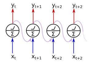
Each recurrent neuron has two sets of weights w<sub>x</sub> and w<sub>y</sub>
