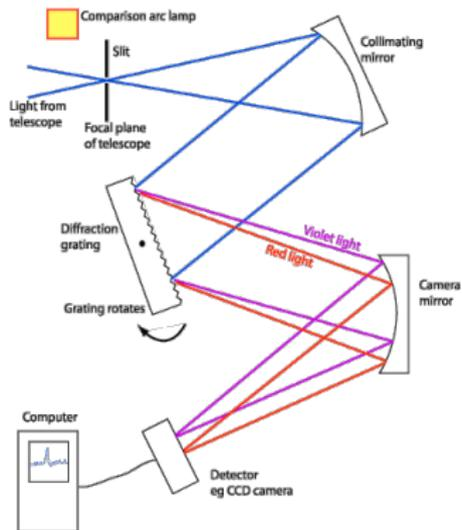
A Schematic Diagram of a Slit Spectrograph
